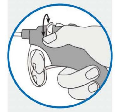
Jaw and shaft rotate 360 degree smoothly.
